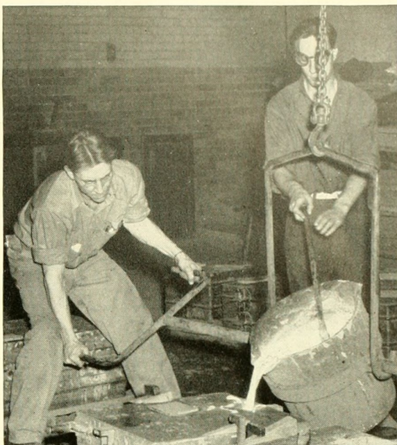
The proper method for pouring molten metal into forms is taught in a class in foundry work at a Detroit vocational school
