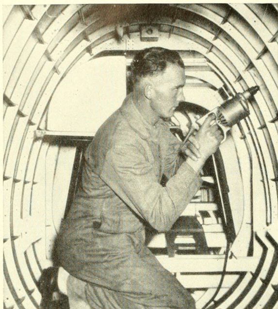
Trainee learning to do a job of drilling inside an airplane fuselage
