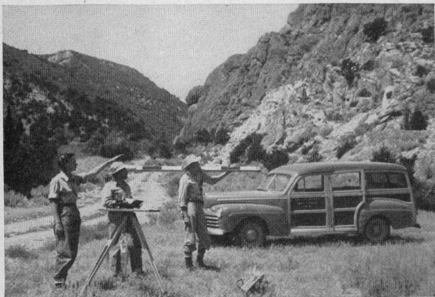
Figure 26.—A geology student on a field trip in Utah mapping at the plane table while her fellow-students do the rod work and note-taking.
