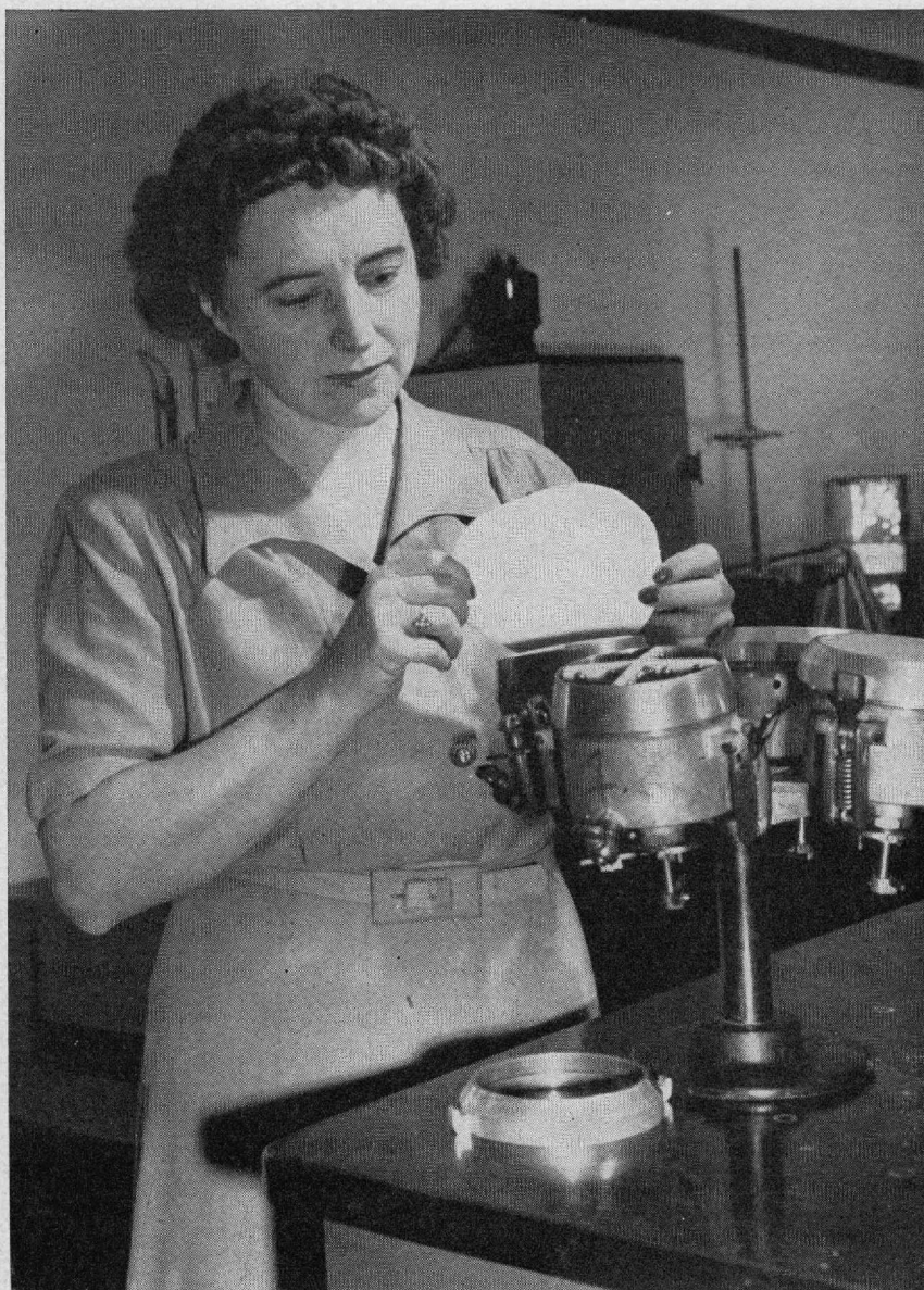
Figure 27.—A chemist, engaged in textile research, preparing to mount a sample of treated cotton fabric for a water repellency test.
