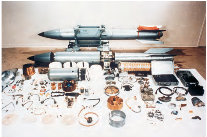
The B-61 bomb, undergoing refurbishment, has approximately 6,000 component parts.
