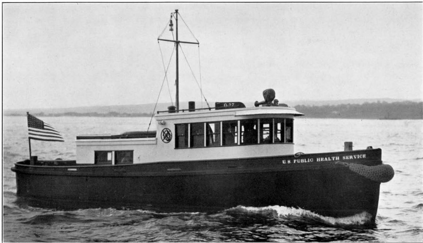
ONE OF THE NEW SMALLER QUARANTINE LAUNCHES (40 FEET) DESIGNED FOR USE AT SMALLER PORTS AND IN SOUTHERN WATERS. It has a 60 h. p. Diesel engine and a welded wrought-iron hull, which will not be affected by dry rot, teredos, or corrosion.
