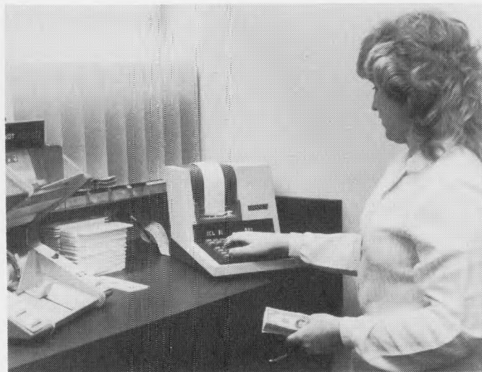
SHERIDAN Bank has positioned the Brandt Model 957 Coin Sorter behind the teller line. This unit sorts and counts up to 600 coins per minute. The Model 957 provides batch totals as well as day-end denomination totals and has programmable bag stops.
