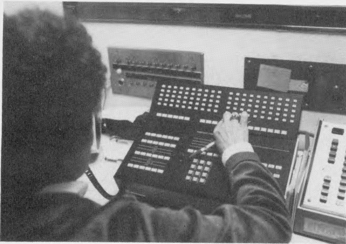
Dimension Communications System is an electronic PBX with a stored program control, offering over 100 features.
