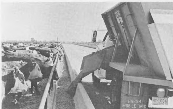
FEED TRUCK with automatic auger system continuously mixes feed rations at Farr Feeders, Inc., Greeley, Colo., with capacity output of 2,100 pounds of fully mixed rations per minute.
