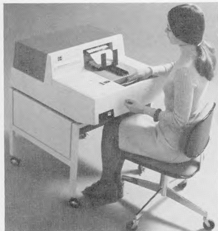
THE RECORDAK Reliant 450 microfilmer can photograph more than 500 check-size documents in a minute at a 40:1 ratio.
