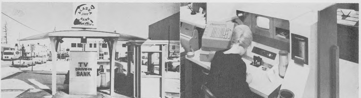
ANCHORAGE, ALASKA installation of the TV Bank Corporation is controlled from the console inside the bank. Customers are viewed through closed-circuit television and transactions handled through pneumatic tubes.
