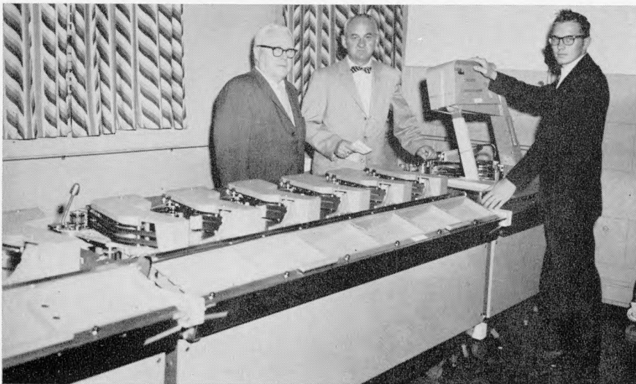
DAILY OPERATION of its check sorter-reader was begun last month by Central National B&T immediately after delivery from the manufacturer, Pitney Bowes National Cash Register. Familiarizing themselves with machine, which will process 750 checks per minute, are (from left): Harold C. Winder, v.p. & cash.; Roger Hicks, transit mgr., and Norman Wilson, asst. transit mgr.
