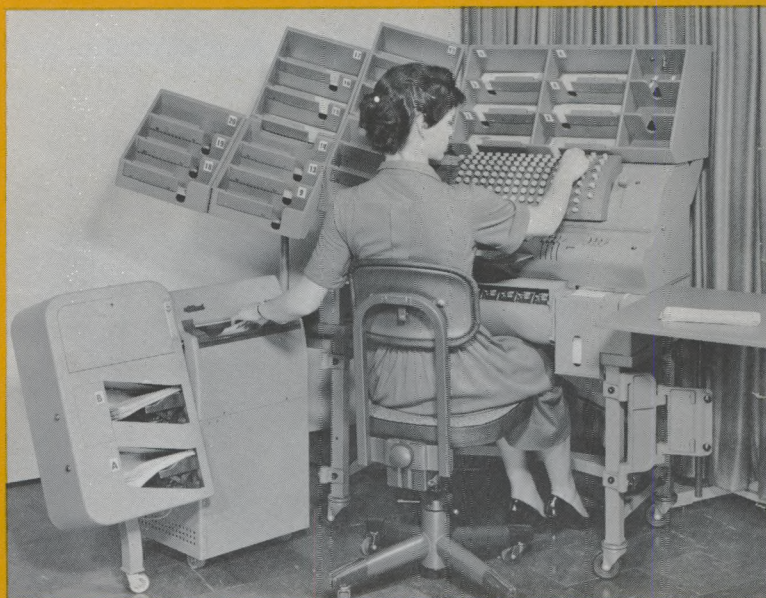
AMOUNT IMPRINTER. Imprints dollar amounts on checks and deposit tickets. This machine may be linked with a proof machine or an adding machine.
