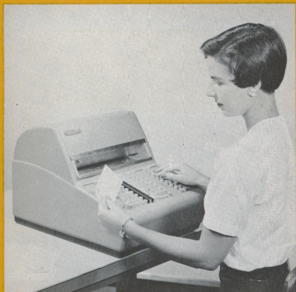
QUALIFICATION PRINTER. Encodes transit routing symbols and account code numbers on unencoded items received by the bank.
