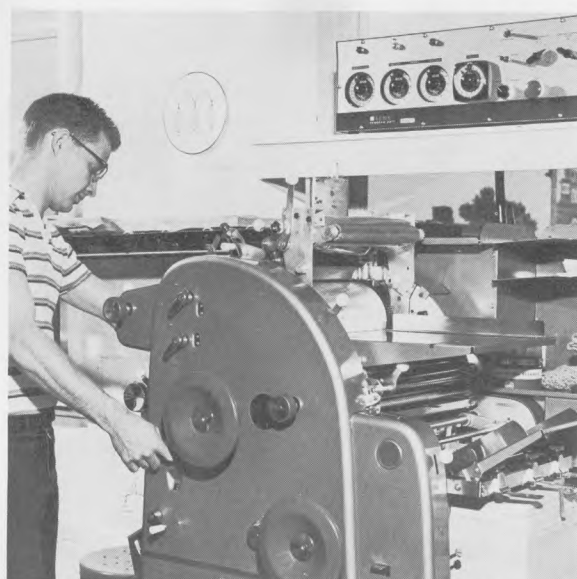
Newest automated offset equipment is used in the magnetic check encoding operation. Checks are pre-lithographed on other Magna-Chek litho presses.
