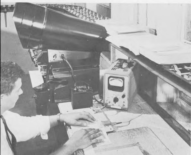
Ultra-modern optical and electronic test and quality-control equipment is essential to first-rate magnetic encoding operation. Magna-Chek imprint is magnified 50 times for image analysis, then electronically checked for signal strength.
