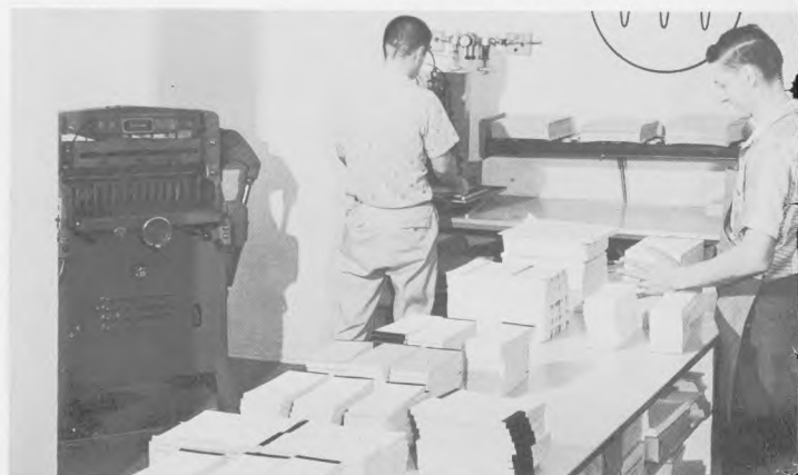
Conveyor delivers encoded checks to semi-automatic stitcher and cutter prior to final assembly and delivery.
