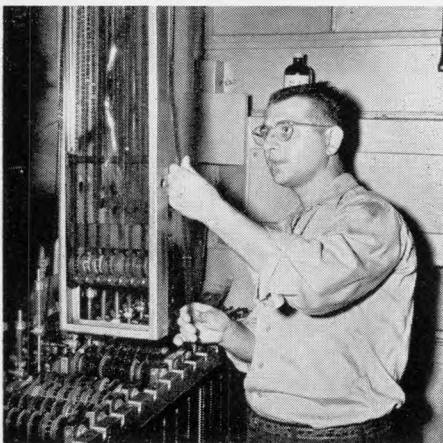
MICROFILM salvaged from flooded areas is passed through the regular washing tanks for final cleaning before drying. G. Disconti checks the film condition in the New York Recordak laboratory.
