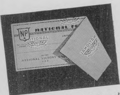
Note how the trade-mark design and wavy lines appear on the back of the check in perfect register with the front. The endorsement is protected as well as the face.
