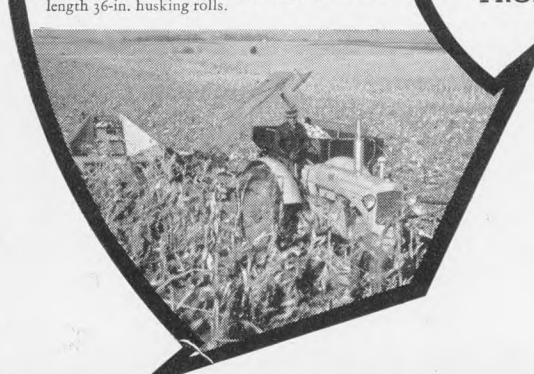
Below: MM Huskor — 2-row corn picker-husker, power-take-off driven from Universal "Z" 2-3 plow tractor. The Huskor has longer picking rolls, 12 full length 36-in. husking rolls.
