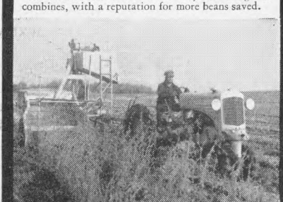
Below: MM Huskor — 2-row corn picker-husker, power-take-off driven from Universal "Z" 2-3 plow tractor. The Huskor has longer picking rolls, 12 full length 36-in. husking rolls.
