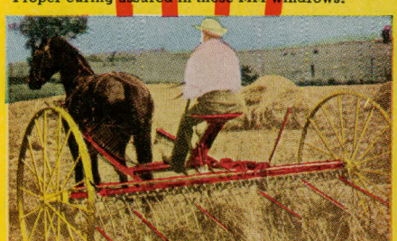
MM Sulky Rake. Modern up-to-date design. Oil tempered, coiled teeth are curved to carry the hay.
