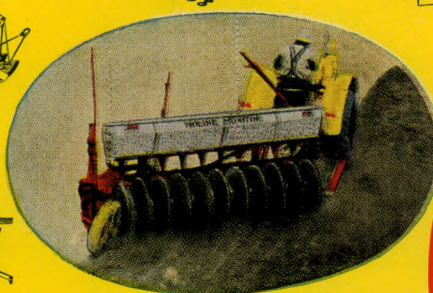
Wheatland Disc Plow with Moline-Monitor seeding attachment.
