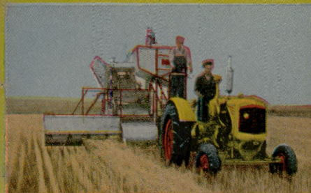
Harvester (12 ft.) with pick-up attachment and the MM Standard "U" tractor harvesting grain from windrow.
