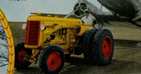
"GT" industrial tractor tows large air liners in and out of hangars.
