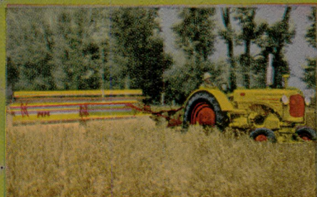
Harvester Windrower and the MM Standard "Z" tractor windrowing a grass crop for curing.
