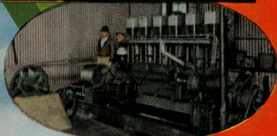
MM 6 cylinder unit engine operating a cotton gin.
