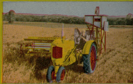
Harvester (6 ft.) with power take-off drive and MM Universal "Z" tractor harvesting standing grain.
