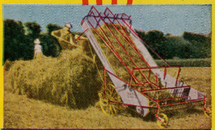
MM Combination Cylinder and Rake Bar Loader. A long life, easy pulling, easy handling loader.
