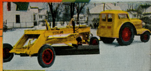
Comfortactor and pull behind type road grader and patrol.
