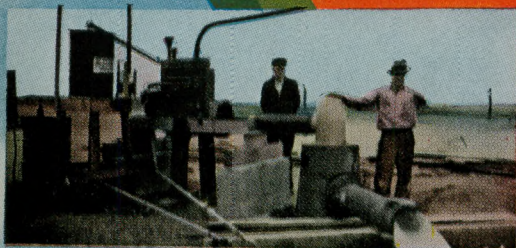
MM 4 cylinder engine pumping water for a large irrigation system.
