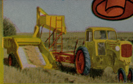
Harvester "69" with pick-up attachment and MM "R" tractor harvesting flax from windrow.
