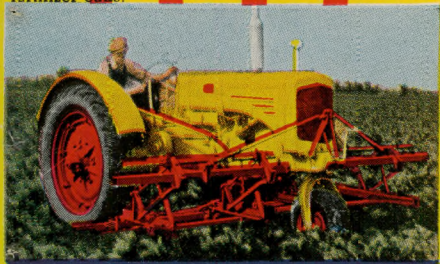
4 row beet cultivator attachment for MM Universal "Z" tractor. Fast, clean cultivating.
