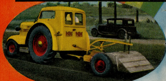
Comfortactor and power take-off driven roto-tiller in operation mixing black-top for road surfacing.
