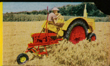
Uni-Mower and Universal "Z" tractor. Backs and turns as part of tractor.
