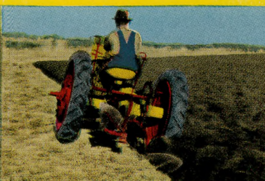
Two way plow for direct attachment to "R" tractor.
