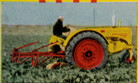
Tractor attached 2 row beet puller attachment for MM Universal tractors lifts the beets carefully without bruising beets.
