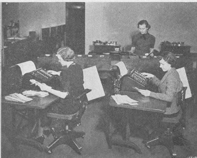
Control totals for the various classifications are quickly summarized here, thus providing a media for accumulating total deposits for general ledger purposes. On these machines, ciphers print automatically, and entire amounts can be written with one motion of the hand—two important factors which contribute much to the speed with which work is done.
