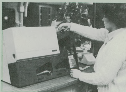
Brandt Model 885 Currency Fitness Sorter sorts currency automatically for 15 ATMs operated by First Security Nat'l, Lexington, Ky.
