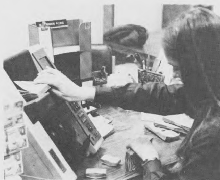
TOP: Liberty Nat'l, Louisville, uses two Brandt cash-settlement systems. Here, currency totals processed on Model 866 currency counter are transmitted to Model 858 central-processing unit. Rebecca Hasting (r.), a.v.p., says bank now can handle more commercial accounts because of acquisition of systems.
