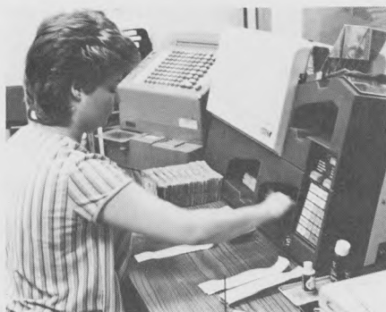
CENTER: Liberty Nat'l processes currency on Brandt Model 866 currency counter, which counts and batches up to 1,500 bills per minute and can be equipped to detect counterfeit bills.
