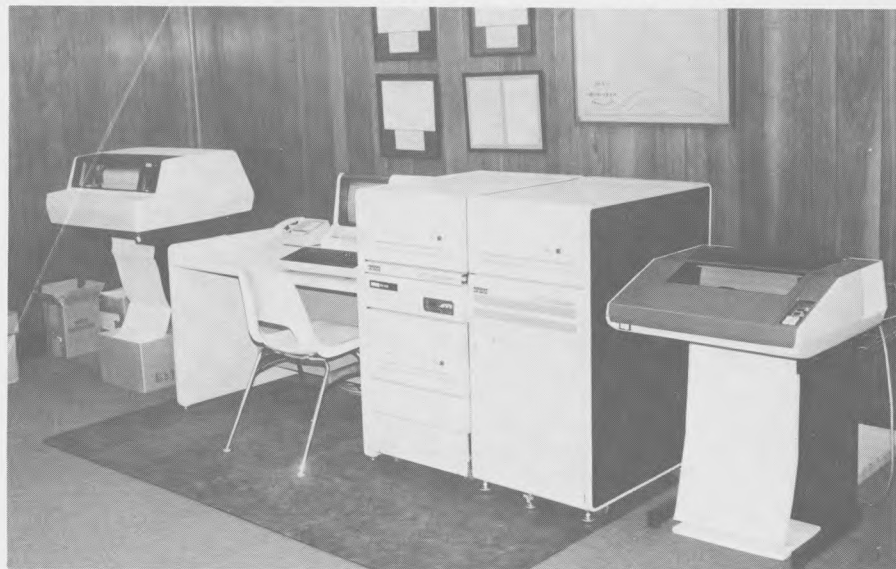
Total Bank Control System at Bank of Augusta, Ark., includes, from l.: printer; desk with keyboard, video screen and telephones; processor with two disc-drives; additional disc drive; second printer.
