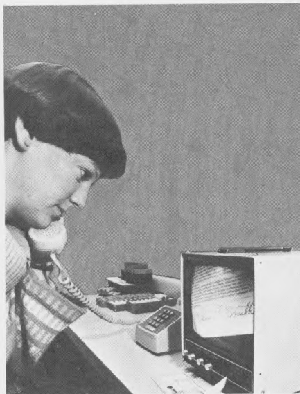
LeFebure, Cedar Rapids, Ia., manufactures this CCTV-based system that can provide instant signature-card display from central point to any station on-premise via coaxial cable.
