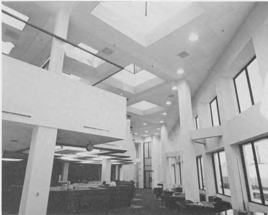
First and second floors extend into 6,000-square-foot triangular-shaped customer-service area illuminated during day by four large skylights.
