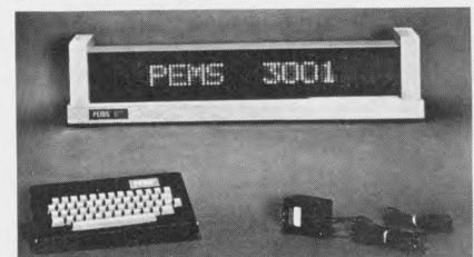
PEMS 3001 display sign (top), programmer (l.) and power pack (r.) make up new One-Up computer sign.
