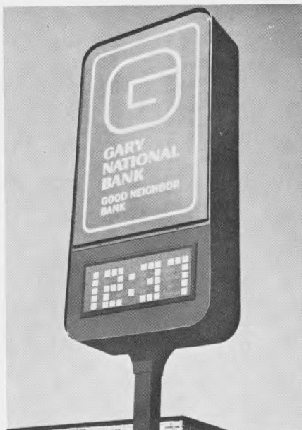
FlipOmatic II time-and-temperature display by Time-O-Matic, Inc., is owned by Gary (Ind.) National. Sign features metal rectangles to form numerals, eliminating light bulbs.
