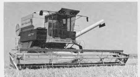
Twin-rotor combine utilizes spinning rotors to thresh and separate grain. Manufacturer — Sperry New Holland — claims twin-rotor process results in less crop damage and loss.
