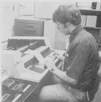
Electronic accounting machine's tape cassette capability is an integral part of on-line communications system linking American State, Charleston, Ark., with computer center 100 miles away in Fayetteville.
