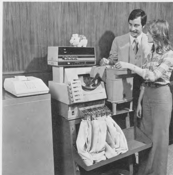
Harry Nedoma, sales rep., Brandt, Inc., checks out new coin sorter/counter with teller at First Nat'l, Peoria, Ill. Bank purchased equipment to eliminate Monday problem of breaking coin wraps and recounting coins brought in by area churches.
