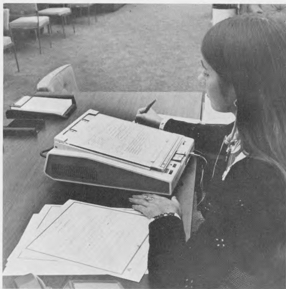
Employee of Fifth Northwestern Nat'l, Minneapolis, uses sound page system to review teller job skills. Unit employs pages that "talk" to employee—back side of each page is coated with magnetic material that holds up to four minutes of sound. Unit is manufactured by 3M Co.
