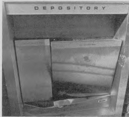
Damaged night depository bears silent witness to futile attempts by burglars to "liberate" deposits from People's Liberty Bank, Fort Wright, Ky. Due to security design of the Mosler Magna Dual Bank and Envelope Depository, even heavy pry bars proved futile in penetrating receiving safe.
