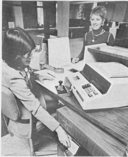
Teller at First Wisconsin Nat'l, Madison, reaches for currency being dispensed by Diebold Accelerated Cash Terminal, which automatically provides exact amount of currency of check being cashed by customer. Coins are handled separately. Use of terminal is said to cut transaction time to 20 seconds per check.
