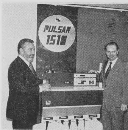
Andre Amiel (l.), pres., Amiel Industries, and Marcel Brisebarre, inventor, pose with AI-1510-Pulsar electronic coin sorter and counter. Machine is said to be able to handle up to 2,000 coins per minute in up to eight denominations.
