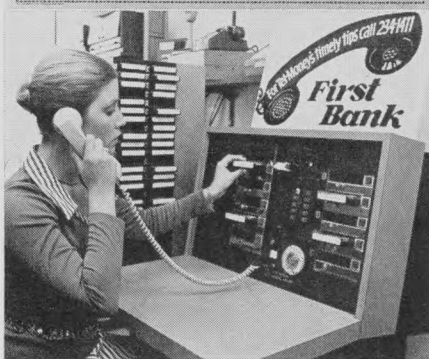
ABOVE: Ad for Tel-Money program of First Bank, South Bend, Ind., tells about service wherein one can call number and hear any of 40 recorded messages on financial matters. BELOW: Operator inserts tape into playback machine. Tape contains message that caller has requested and if caller needs additional information on topic, tape instructs caller to phone bank's personal service rep.
