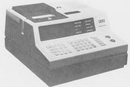
This NCR 279 unit will be installed at each teller station at Kentucky Group banks to permit entry to on-line EFT system, cut transaction times.
