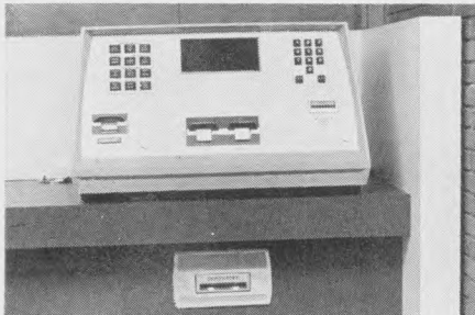
This is Docutel "tabletop" ATM being used by Liberty Nat'l, Louisville, in two Main Office locations and at its Airport Branch. Units complete most transactions in seconds, provide cash in increments from $5 to $100.
