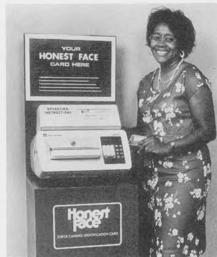
This is Honest Face check-cashing terminal being offered by First National, Atlanta, for use in local food stores. Customer inserts card, punches secret code, selects type of transaction, inserts check, and machine verifies or prohibits transaction in about 30 seconds. System is offered in most major grocery chains in area, is said to lower overheads through reduction of returned checks, faster check-out lines.
