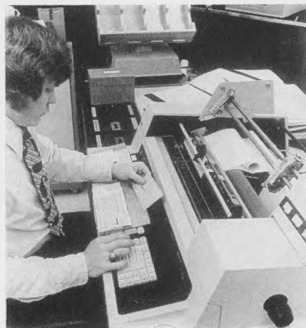
LEFT: Nolan Glass enters master file changes onto magnetic tape through NCR 399 Accounting Computer. Machine is used off-line for accounting functions, including writing customer payrolls and accounts receivable, and it also functions as on-line terminal over leased phone wires to main-frame computer in Houston.
