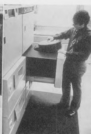
SECOND FROM RIGHT: NCR Century 200 system contains central processor with 64,000 characters of memory, as well as four NCR 657 magnetic disk units, each of which is capable of holding 56 million characters in memory for operating CIF systems. RIGHT: CIF reports are printed out on 1,500-3,000-word-per-minute NCR printer.
