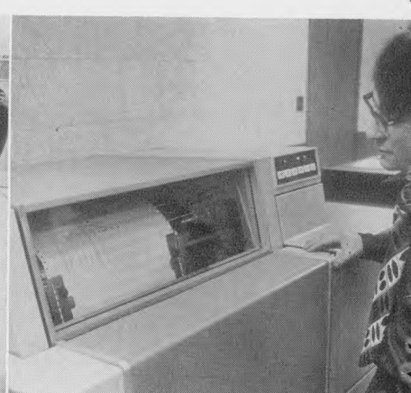
SECOND FROM RIGHT: NCR Century 200 system contains central processor with 64,000 characters of memory, as well as four NCR 657 magnetic disk units, each of which is capable of holding 56 million characters in memory for operating CIF systems. RIGHT: CIF reports are printed out on 1,500-3,000-word-per-minute NCR printer.
