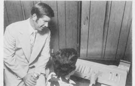
Walter Hinkle, operations vice president at Hancock Bank, watches bank's operator use 812A PBX console. New equipment has enabled bank to cut its operator staff in half.
