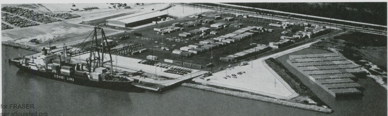
Ship at left is unloading containerized cargo at Port of New Orleans while barges at right await loading on decks of ships that will carry them to foreign ports where they will proceed to destinations via rivers.
