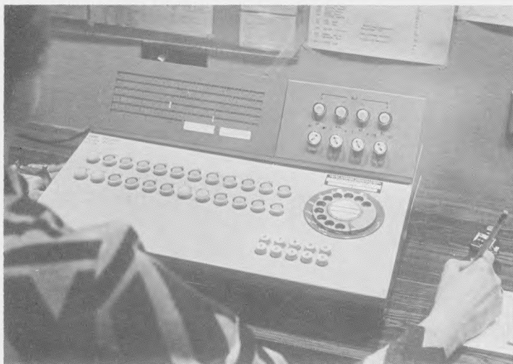
LEFT: This electronic console is heart of telephone system installed at Glenview (Ill.) State by United Business Communications. On it operator answers calls to bank and to Cummins-Allison Corp., affiliated firm
