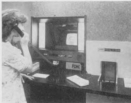
To transact business via Personal TV Teller, customer talks to teller on phone, if private conversation is desired, deposits transaction materials in captive carrier, pushes button, and materials are on way to teller via pneumatic tube. Teller completes transaction and returns materials in same manner.
