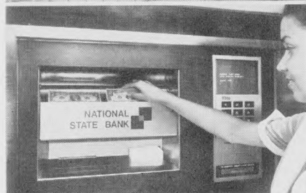
Diebold "TABS" 500 is activated by bank card which causes transparent vandal shield to recess. Customer keys in four-digit code and follows instructions on illuminated panel.
