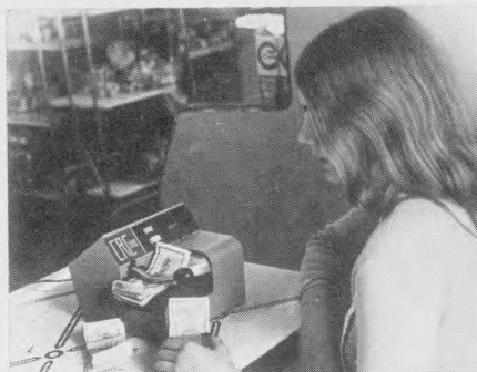
CRC-300 currency and food stamp counter attacks stack of food stamps that were formerly counted manually. Automatic device enables teller to perform other duties during counting time.
