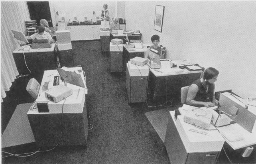
Overall view of word processing center at First of Little Rock. Five magnetic tape "Selectric" typewriters are along right wall and in left foreground. At left rear are two magnetic tape composers. Four telephone recorders are across back wall and a transcribing unit is on each magnetic tape unit.
