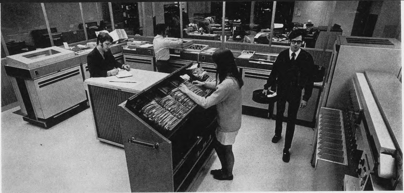
Creve Coeur Bank's central information file data is processed by this NCR Century 100 computer, installed in late 1969. From left: EDP Systems Manager Robert W. Hodge fills out the production schedule, an operator places punched cards in the reader, another prepares
