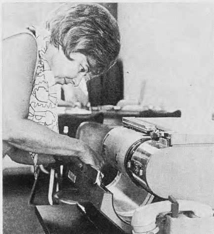
Facsimile transmission device transmits loan applications or other information from branch to head office for decision-making.
