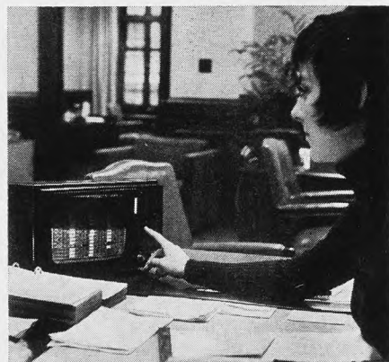
Members of the bond department, Continental Bank, Chicago, now receive televised market quotations at their desks by means of closed-circuit TV. Six ceiling-mounted cameras transmit up-to-the-minute market information from wall-size quotation boards to receivers at desks in other rooms. When someone needs a quotation, he presses one of six buttons on his desk-top receiver and scans the screen for the price he wants.
