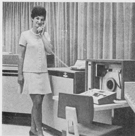
Data transmission from magnetic tape unit of NCR 720 Remote Bank System is made over regular telephone lines. Operator is shown here establishing phone connection prior to transmission.
