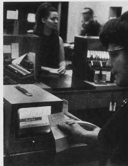
console and in seconds signature card is displayed on reader screen and on TV monitor. Operator then punches button to send TV image to teller requesting verification (right photo).
