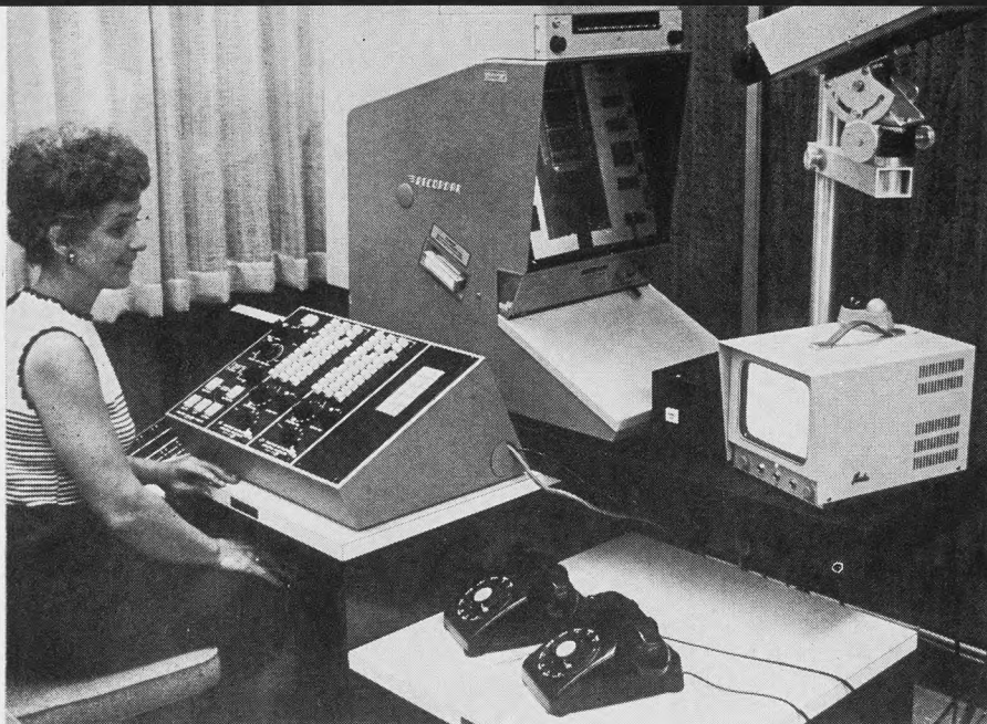
Operator in retrieval setup in bank's operations center (left photo) selects magazine from file to her left for insertion into Recordak reader-printer. She keys in customer's account number on control
