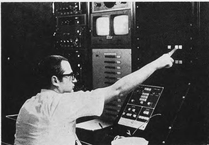
Operator presses button on control panel located in master control room of new Management Communications Center at First National, Chicago. The panel controls closed-circuit television for graphic presentations which are transmitted to offices of bank's two senior officers. Programs can be controlled either by operator here or by the officer himself through a control panel in his desk drawer.
