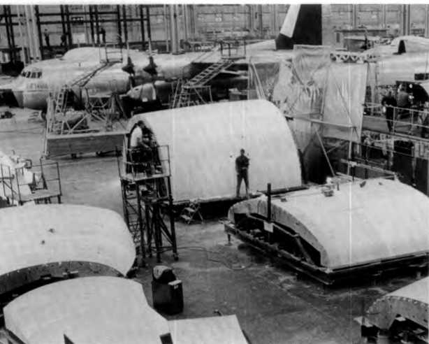
Master models for the world's largest plane, the C-5A, lie next to production lines for the C-130 Hercules and C-141 StarLifter.
