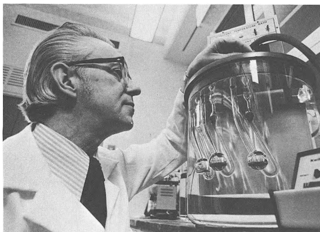
The Association of Petroleum Re-refiners is supporting an Industrial Research Associate to work with Bureau scientists on an oil recycling program. This associate is determining the viscosity of some recycled oil.
