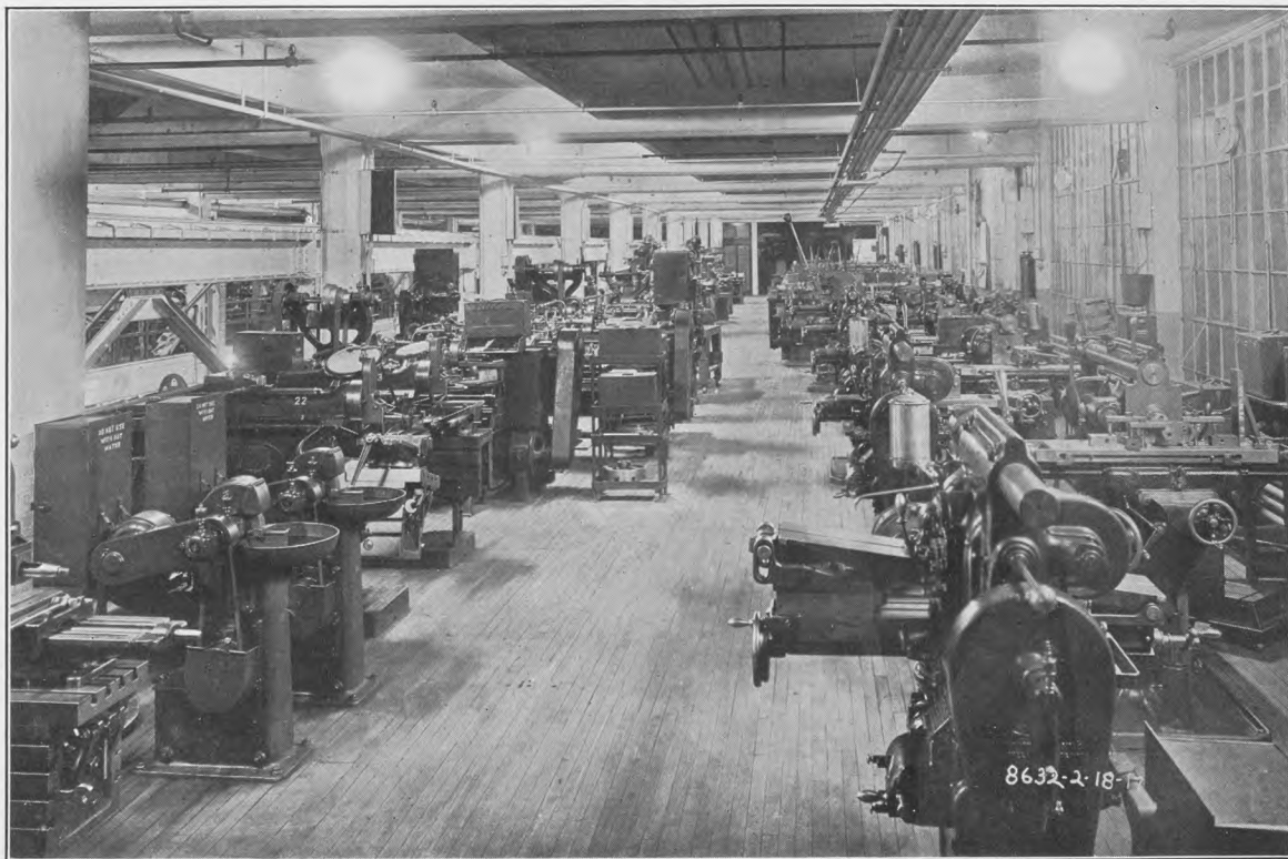
PLATE VIII.—MACHINE SHOP. AT LEFT, ROUGH HAND GRINDING; AT RIGHT, MILLING MACHINES.
