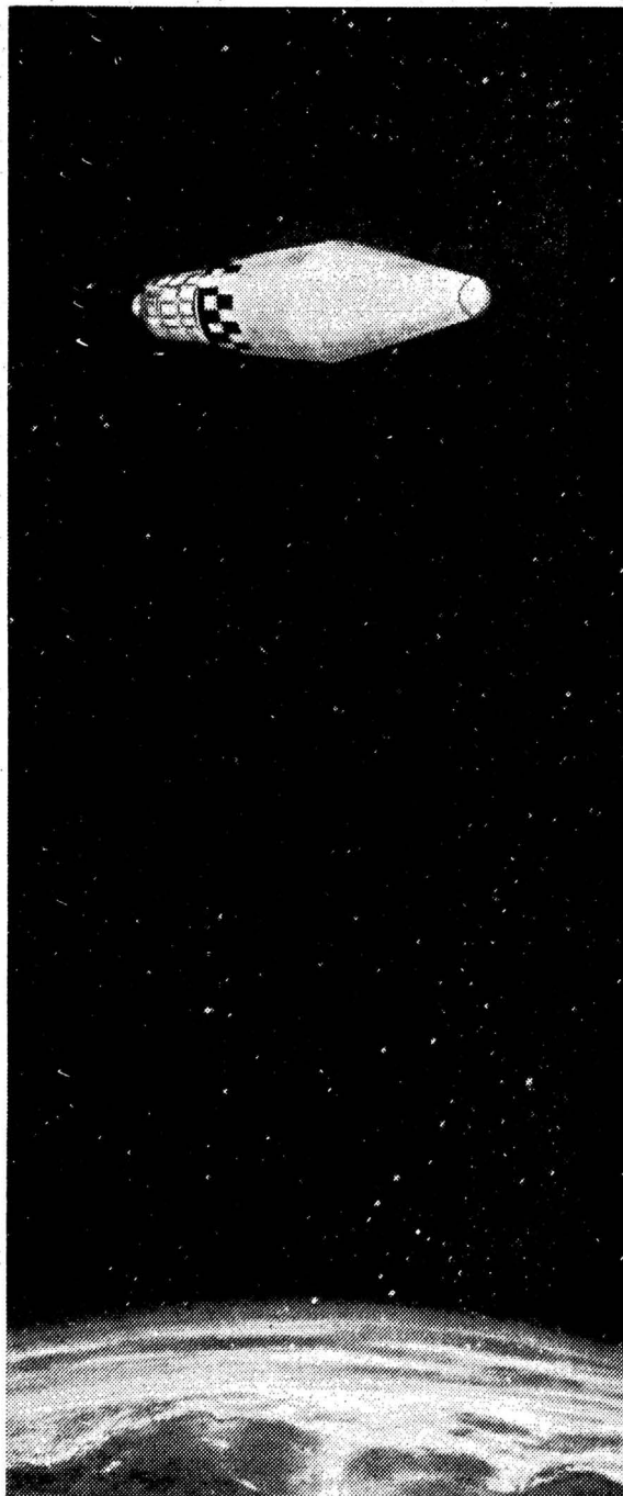
Once in orbit, the Agena satellite radios back to its tracking stations more than a hundred measurements of its performance and of the conditions it encounters as it circles the earth at 18,000 mph.
